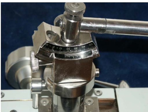
FIG. 7. (Color online) Angle adjusting device mounted horizontally. The coupling holder for the laser handpiece can be rotated in any direction.
