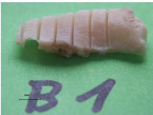
FIG. 11. (Color online) Macroscopic assessment of sample B1, double path with the same program. Note no carbonizations, exact repassing in the same cut, thus only deepening the cut without damage to the incision walls.
