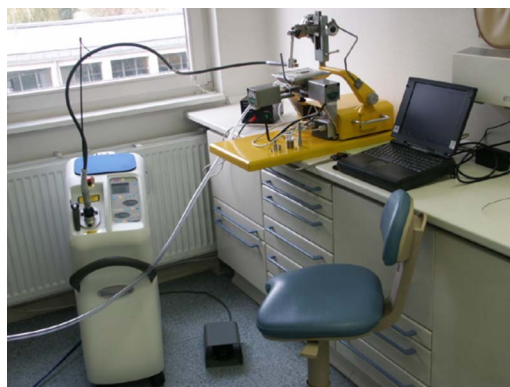
FIG. 9. (Color online) Fully mounted mechanical experimental setup, including electronic control, power supply, and control card.
