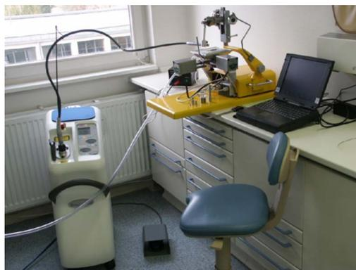
FIG. 9. (Color online) Fully mounted mechanical experimental setup, including electronic control, power supply, and control card.
