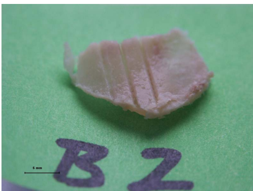
FIG. 10. (Color online) Macroscopic assessment of sample B2; from left to right: 1 mm/2 s, 1 mm/3 s, and 1 mm/4 s. No carbonization and constant incision depth and width along each preparation line.
