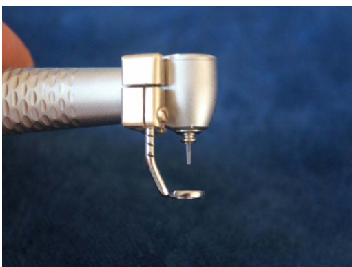
FIG. 1. (Color online) Constructed and fixed calibration unit on the laser handpiece to be used (total view). Handpiece, angle 90° (Millennium Waterlase, Biolase Technologies, San Clemente, CA, USA).
