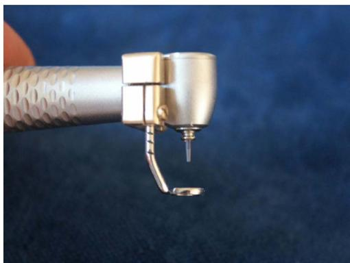
FIG. 1. (Color online) Constructed and fixed calibration unit on the laser handpiece to be used (total view). Handpiece, angle  $90^\circ$  (Millennium Waterlase, Biolase Technologies, San Clemente, CA, USA).
